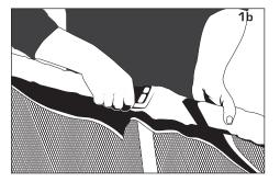
Step 1b: Work the sail down the mast from midway along the sleeve.
